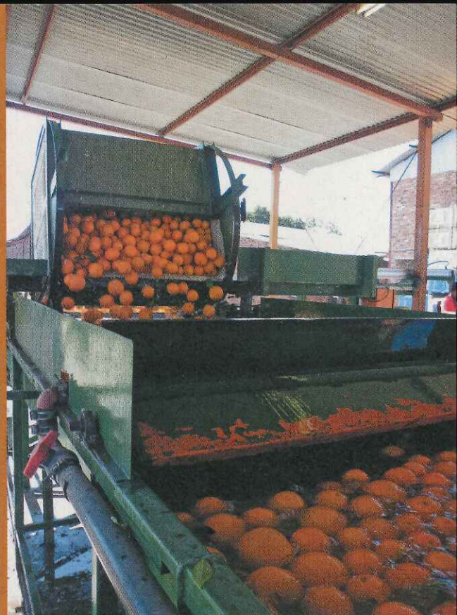
ABOVE: Stefan, a mechanical engineer by training, designed and built this tipper that tips bins and performs the first wash of fruit from the orchards. It cost less than R100 000, compared with up to R700 000 for a new one.
